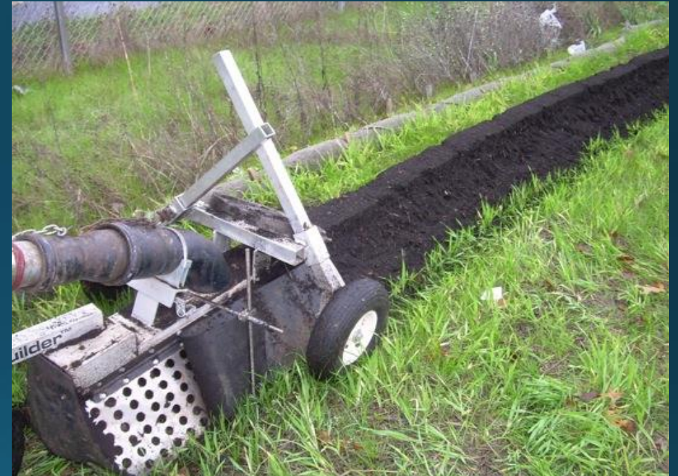
Application using a side discharge spreader with a berm attachment.
