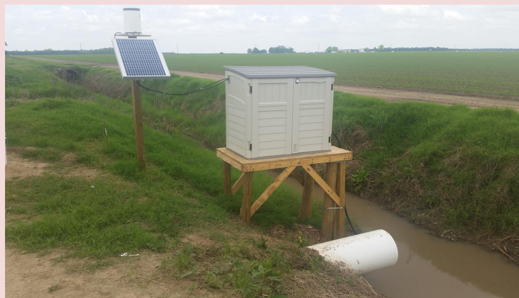
Fig. 1 An ISCO 6712 Automatic Sampler is installed at all sites to automatically collect water samples once the threshold water flow is detected. Each monitoring station was equipped with a flow outlet structure (the open-channel pipe in the current situation). The outlet structure was outfitted with flow sensors, data loggers, and communication devices.
