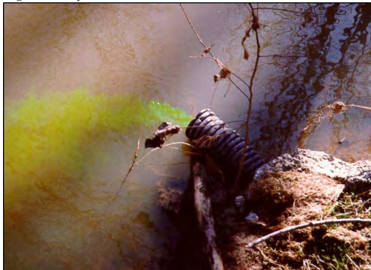
Figure 15: Dye at outfall location
