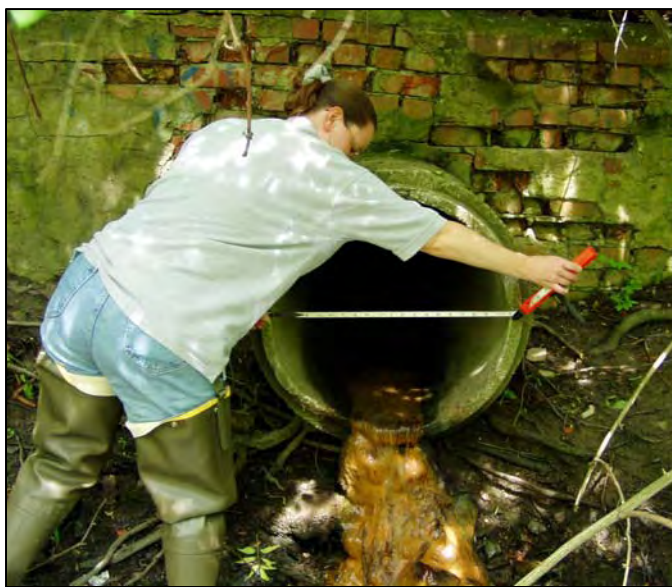
Figure 9: Measuring size of outfall
