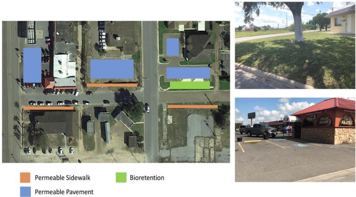
Figure 9. Proposed BMP implementation and location for Site #3
