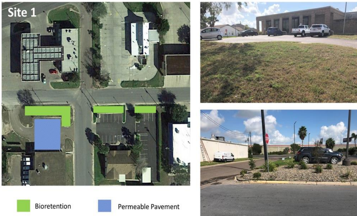
Figure 7. Proposed BMP implementation and location for Site#1
