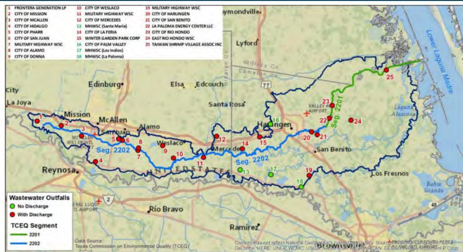
Figure 5.2. Permitted wastewater outfalls within the Arroyo Colorado watershed
