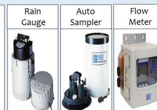
Figure 5: Monitoring equipment to measure rain stormwater runoff volume and collecting samples.
