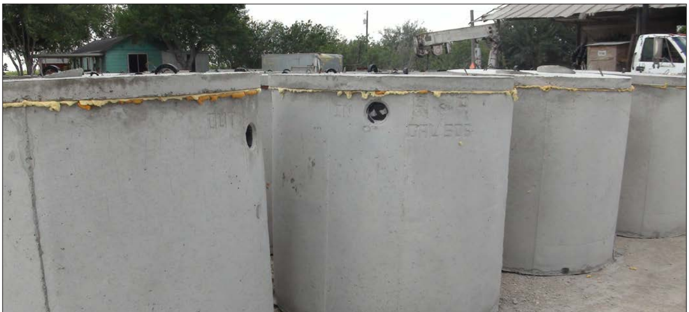
Newly constructed 500-gallon septic tanks
