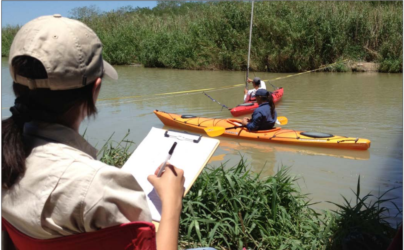
UTB/UTRGV students measuring streamflow at Cemetery Road crossing
