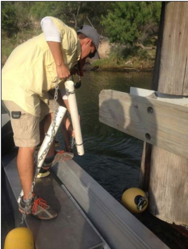
A UTB/UTRGV student deploys a continuous sampling water quality sonde near the Rio Hondo bridge in the Arroyo Colorado.
