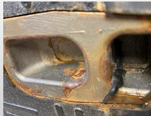
Other Composite Cover shows post-process machining of the fastener holes. Glass Fiber can be seen exposed.
