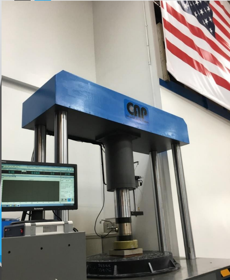
Photo Show CAP's Onsite Proof Load Test Equipment
