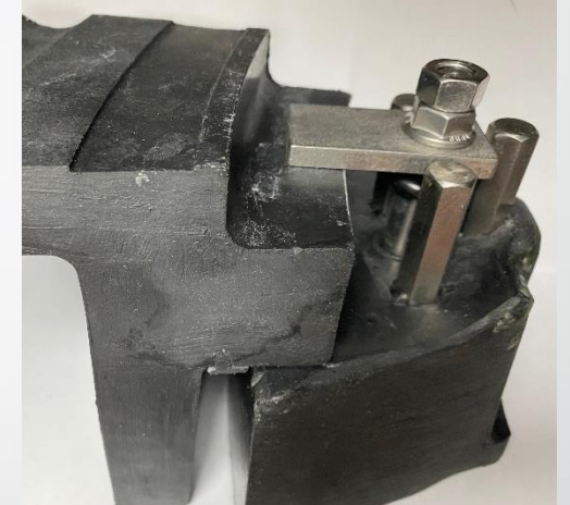
Paddle Locked Secured w Pins
