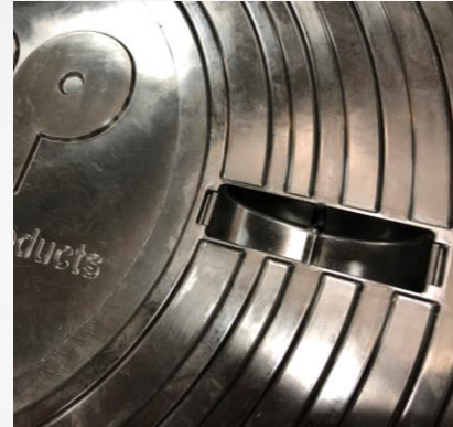
CAP Molds-in Features Protecting Fiber
